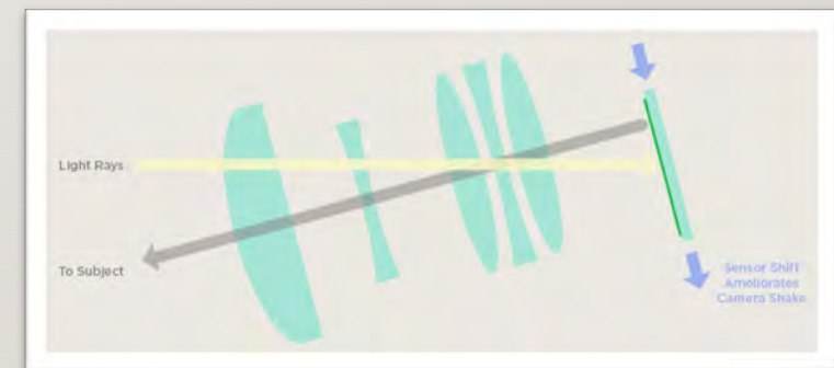
In-body - physically shift the image sensor to compensate for camera body movements
